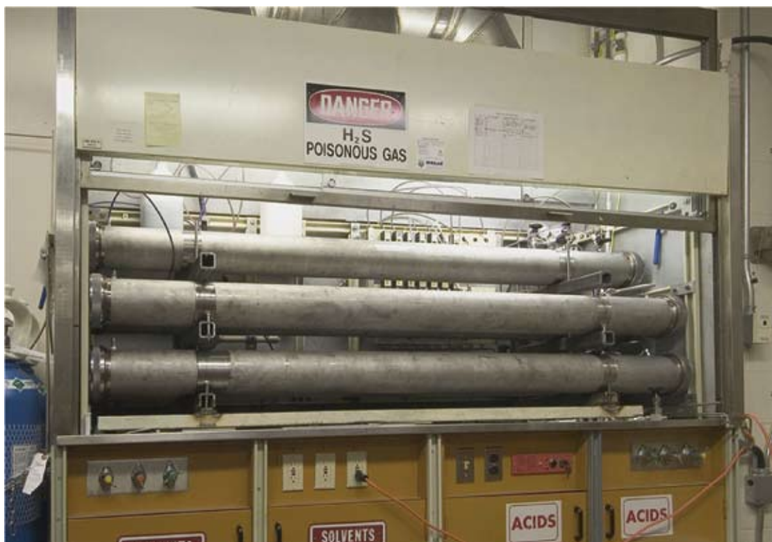
Fig. 1—Sour immersion cells for CT bend-fatigue specimen pre-exposure.
